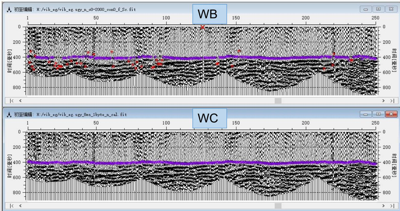
Inverting the model by tomography (down), by refraction(up)
